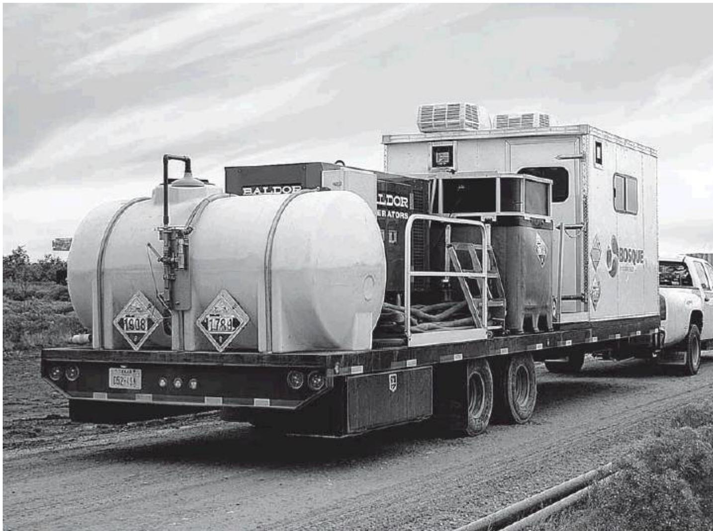
A Bosque Systems LLC Dionix mobile unit cleans water from oil operations, reducing the need for freshw sources and for disposing water deep underground. [
